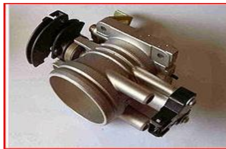
Fig. Throttle body showing throttle position sensor. The throttle cable attaches to the curved, black portion on the left. The copper-coloured coil visible next to this returns the throttle to its idle position when the pedal is released.
